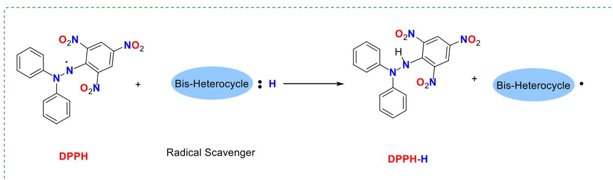
**Figure 2.** Reaction mechanism of 2,2-diphenyl-1-picrylhydrazyl (DPPH) with antioxidant.
