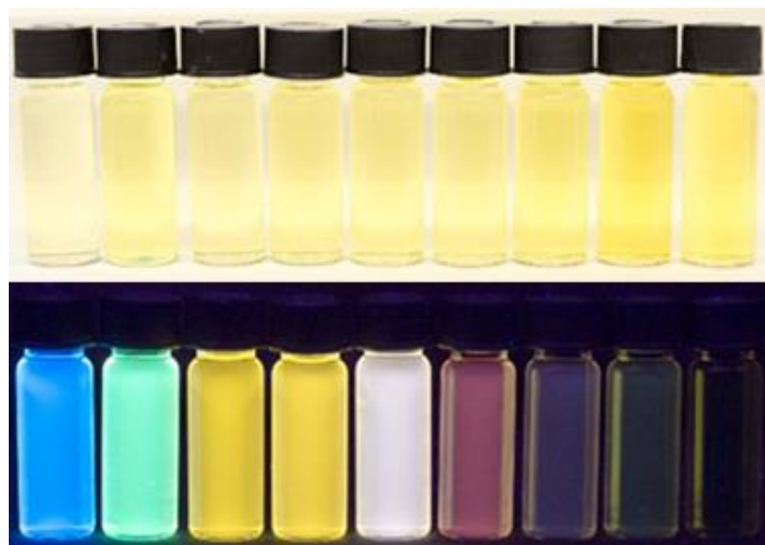
Figure 2. Dye MEQDMA ( c(\text{MEQDMA}) = 10^{-4} M, T = 293 K) in daylight (top) and fluorescence (bottom) with variable solvent polarity (from left to right: cyclohexane, toluene, tetrahydrofuran, ethyl acetate, dichloromethane; acetone, acetonitrile, isopropanol, methanol; \lambda_{exc} = 365 nm, hand-held UV lamp).
