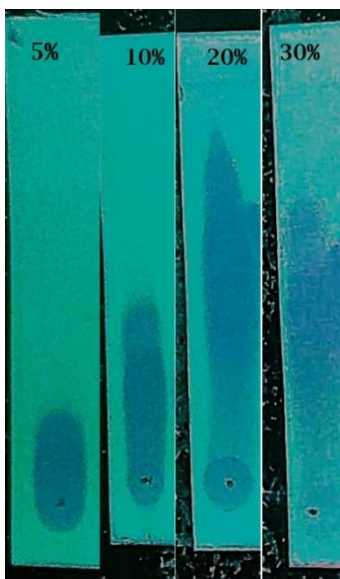
Figure 3. TLC fingerprints of the enriched fraction of Commiphora mukul in 5, 10, 20, and 30% EtOAc: Hexane solvent system (UV visualization).
