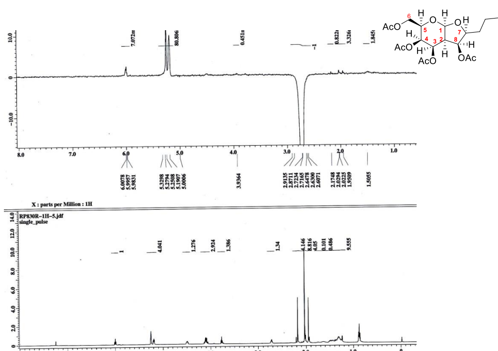
Figure S 27. nOe spectrum of compound 26 for irradiation of H-2.
