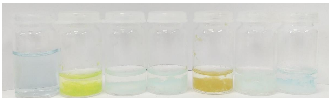
Figure S 50. From left to right: methylene blue solution (3 mL, 4\text{ mgL}^{-1} ) without gelator, gelators 1, 4, 5, 6, 7, 8 (10 mM), gelled with HCl, within 12 hours after addition of methylene blue solution (3 mL, 4\text{ mgL}^{-1} ).
