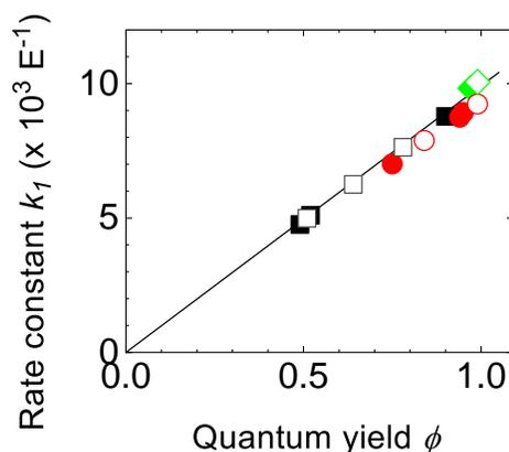
**Figure 5.** Correlation between the rate constant and quantum yield for  $^1\text{O}_2$  generation. Solvent: MeOH (■, □),  $\text{CH}_2\text{Cl}_2$  (●, ○), toluene (◆, ◇). Light source: 395 nm LED (■, ●, ◆), 525 nm LED (□, ○, ◇).
