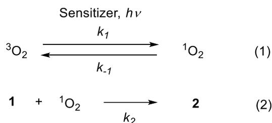
**Scheme 3.** Elementary reactions for the ene reaction of **1**.
