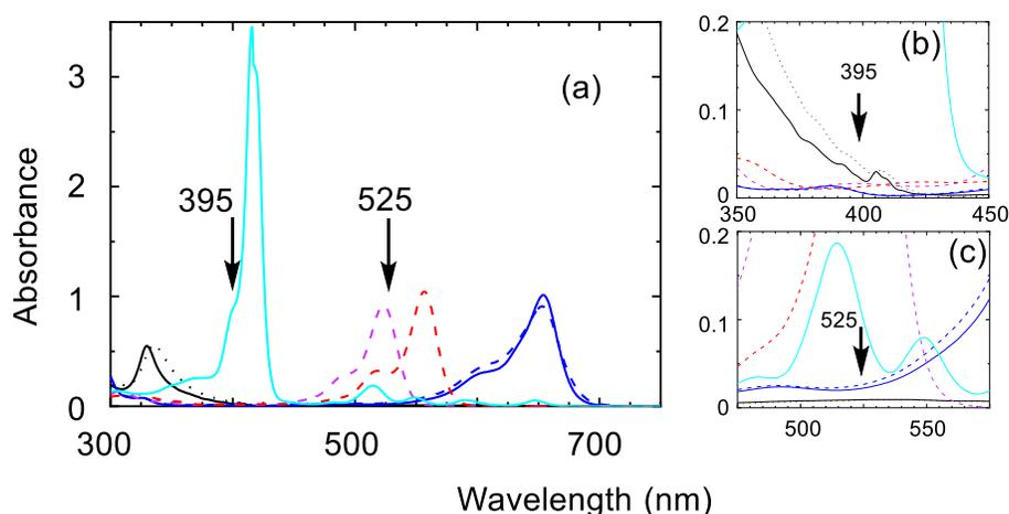
**Figure 1.** (a) UV absorption spectra of various sensitizers in different solvents. The wavelength at 395 and 525 nm are also shown in the figures. The concentration of the sensitizers was: (a)  $1.00 \times 10^{-5}$  M and (b, c)  $1.00 \times 10^{-4}$  M in  $CH_2Cl_2$  (—), MeOH (- - -), and toluene (.....). Sensitizers: **MB**, blue; **EY**, violet; **RB**, red; **TPP**, light blue;  $C_{60}$ , black.
