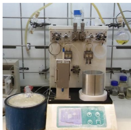
Figure 1. Uniqsis FlowSyn SS reactor set-up for the synthesis of aryldiazonium tetrafluoroborates.
