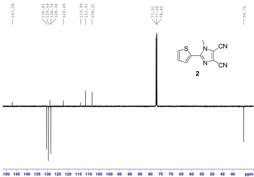
Figure S2. 13 C-NMR APT (125 MHz, CDCl 3 , 25 °C) spectrum of compound 2.
