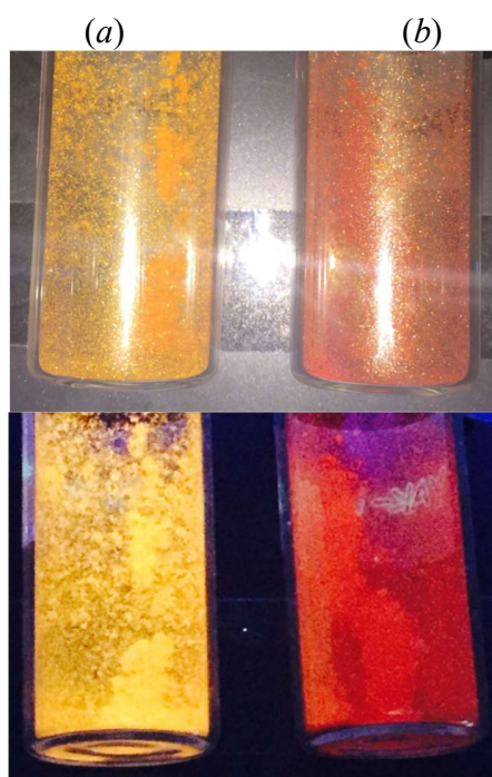
Figure 8. Photographs of (1) compound 20d and (2) compound 21d under daylight ( top ) and under UV irradiation ( \lambda_{\text{ex}} 365 nm) ( bottom ) in the solid state.
