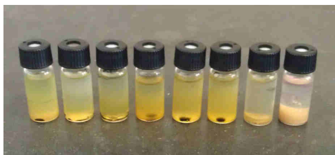
Figure 3. Formation of a precipitated polymer from the reaction of monomer 6 and 4-(aminomethyl) piperidine 27 . Aliquots taken from the polymerization reaction over time. From left to right, aliquots from 0.5 h, 1 h, 1.5 h, 2 h, 2.5 h, 3 h, 12 h, 24 h time points are compared.
