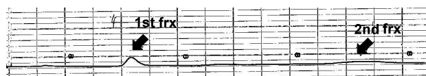
Figure 7. Preparative HPLC with a chiral stationary phase column (Daicel CHRALFLASH-IF, MeOH eluent, 210 nm det.).
