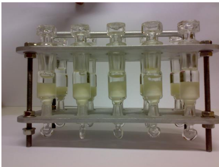
Figure 1. Monolith-filled glass cartridges (20x10 mm i.d.) for high-throughput screening.
