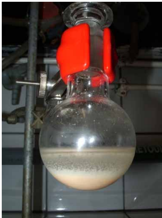
Figure 2. Treatment of the crude Biginelli reaction mixture 7 with deionised water: the upper aqueous layer contains excess of urea or thiourea 6 and the ionic liquid phase bound 3,4-DHPM 7 is insoluble.
